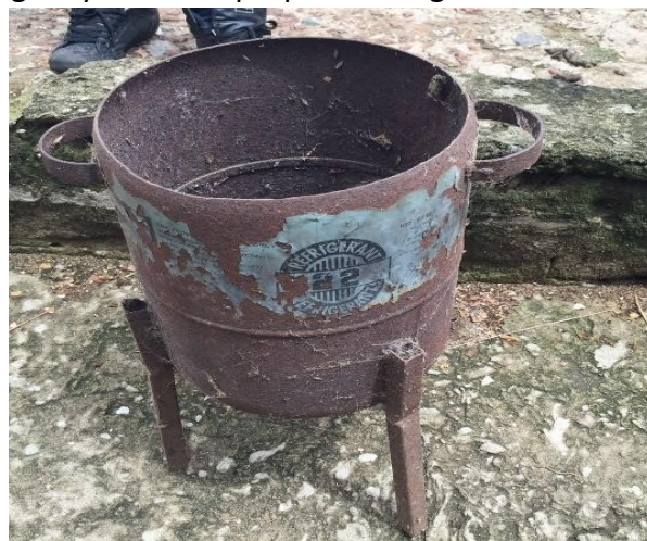
Locally constructed coal pot from empty gas cylinder for proper heating
